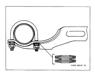
To renew the rear muffler, place rear muffler with socket joint exactly over removed system and mark pipe length of new muffler at the removed system.
