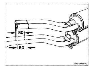
Do not tighten the flange joint to the exhaust manifold until the complete system is attached in the rubber rings. Ensure that the front exhaust pipe is correctly located. Tightening torque of bolts 20–25 Nm.
