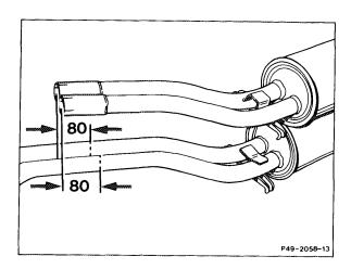
Do not tighten the flanged joint to the exhaust manifold until the complete system is attached in the rubber rings. Ensure that the front exhaust pipe is correctly located. Tightening torque of hex. bolts 20–25 Nm.
