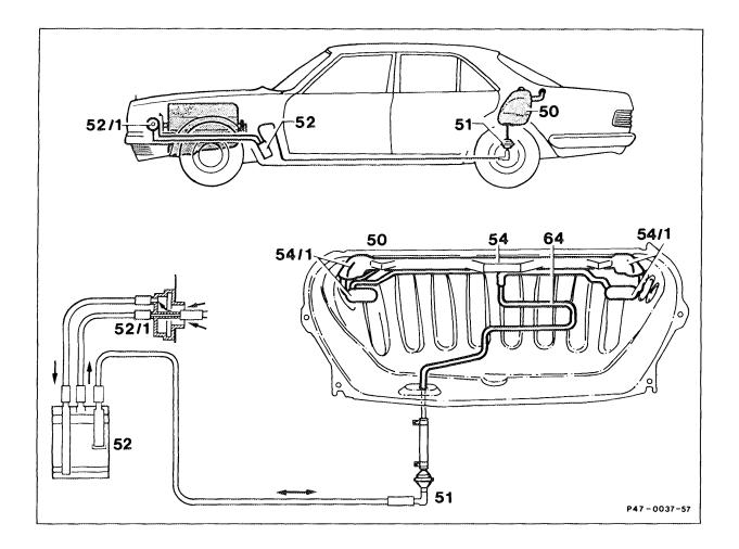
The ventilation system consists of a central pipe (54) with interrupter vessels (54/1). The interrupter vessels (54/1) prevent fuel escaping along the vent line (64). The vent line (64) runs from the central pipe to the vent valve (51). Air is admitted to, and released from the fuel tank (50) through the charcoal canister (52) and the boot (52/1).
