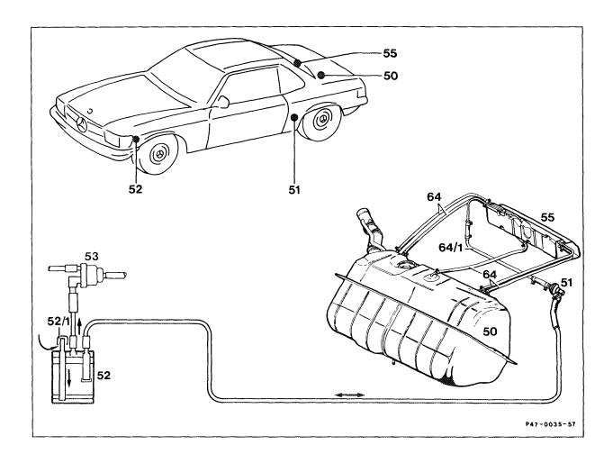
A separate fuel expansion tank (55) is located above the fuel tank which is connected by five lines (64) to the fuel tank. Depending on the fuel level and temperature in the fuel tank, these lines act as overflow, discharge or vent lines
