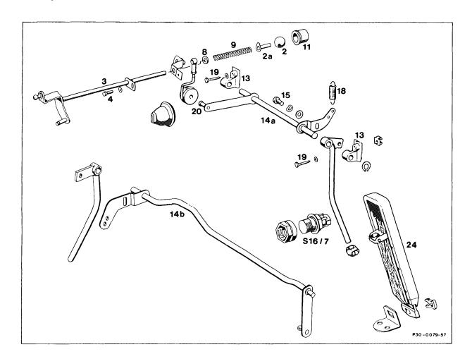
Connecting link with damping ring (20) ... press off lever of accelerator control shaft (14a) (14b, not used), press on.
