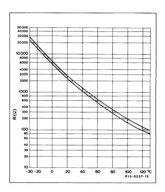
Diagram of 4-pole coolant temperature sensor (EZL/CIS-E), (B11/2)
