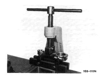
10 Check offset of connecting rod bearing bore relative to connecting rod bushing bore and correct if necessary.
