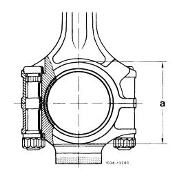
When renewing connecting rods, pay attention to differences in weight of connecting rods.
