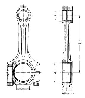
9 Align connecting rod bore relative to connecting rod bushing bore (parallel alignment).
