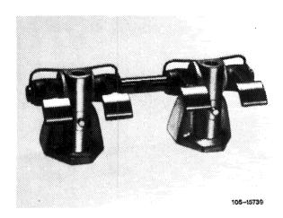
3 Draw tension spring (57), bearing brackets (65) and rocker arms (59) off rocker shaft (58).
