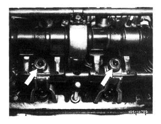
2 Force tension springs off rocker arm brackets.
