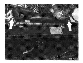
5 Unscrew fastening screws (arrow) for viscofan clutch and remove viscofan clutch with fan together with fan shroud.
