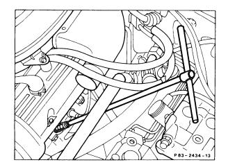
Spark plug connector . . . . . . . . . . slacken by turning to left and right and pull off, fit on. Blow out recesses with compressed air.
