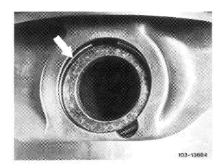
11 Position piston ring clamping strap and introduce pistons into cylinder bore with arrow in the direction of driving.
