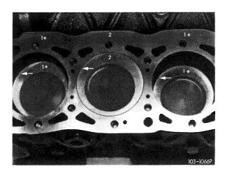
In the event of repairs, hone cylinder bores according to the dimensions of the existing pistons plus the piston clearance (see table).
