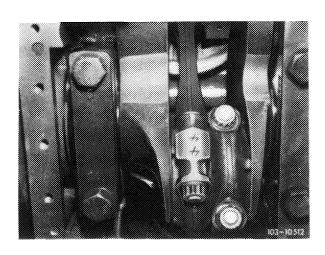
14 Measure distance between piston crown and crankcase mating surface with the piston at TDC
