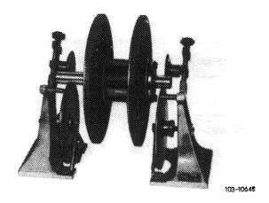
4 Any unbalance can be corrected by drilling holes in the "heavy" side of new flywheel until both flywheels stop at any position without swinging backward or forward.
