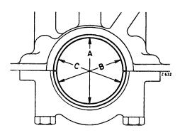
Note: To check the conicity of the bearing bores, measurements are made at the front and rear in bore. If the permissible out-of-round of 0.01 mm in direction "A" is exceeded, the excess dimension on the bearing cap can be removed by carefully applying fine emery cloth. Place emery cloth on surface plate for this purpose.
